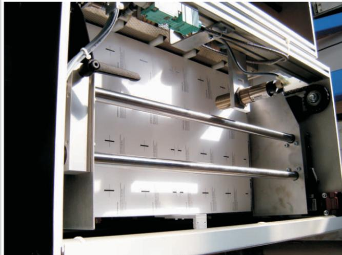
The **ecojet** digital print system is based on the single pass inkjet principle. Latest inkjet technology of Xaar with dynamic print heads offers an optical resolution of 1000 dpi. A high-capacity ink supply guarantees a continuous production. The awarded software solution with all possibilities of color management ensure a HighEnd- quality of the print results.
